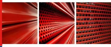
(generally 75mm concave) incorporating either a plastic endlock or a zinc alloy die cast end-lock riveted in position. Wind anchor locks may be fitted on larger shutters. The lath can be 18, 20 or 22 swg as standard or any other gauge if requested. The curtain is supplied with solid lath as standard. Optional extras include perforated or punched "brick bond" lath. Insulated laths are also available offering aninsulated shutter variant with a U value of 4.5W/m<sup>2</sup>K.
